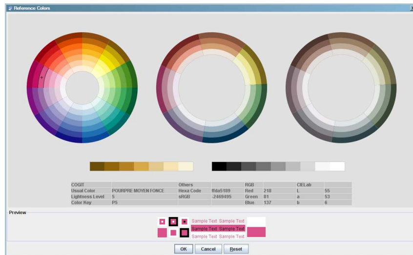
Figure 15 : Chromatic wheels, the COGIT color reference system
